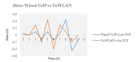
Figure9: Jitter - Wired VoIP VS VoWLAN
