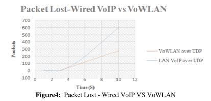
The packet loss is significantly more for wired than for wireless under the UDP protocol. This does not match the theoretical results, in which the instability of wireless packet transfers will result in higher packet loss. This result is due to the queuing type of the duplex links, as there are three separate queues between sender and receiver, which results in undesired queue stacking characteristics resulting in significant amount of packet loss over long periods of times.
