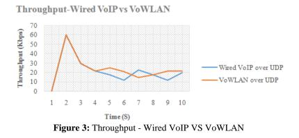
The resulting throughput between wired and wireless VoIP networks under UDP is similar. This is due to the mobile nodes being placed relatively close to the Access Points, so that the signal is strong enough to mirror a wired connection. As seen from the figures, without any background traffic, both VoWLAN and wired networks easily reach the throughput of 60kbps, guaranteeing reliable voice traffic between the clients.
