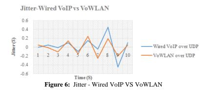
As mentioned in the latency test, the jitter is higher for the wireless network than for the wired. This is also theoretically correct, as wireless signals are prone to interference and signal instability.
